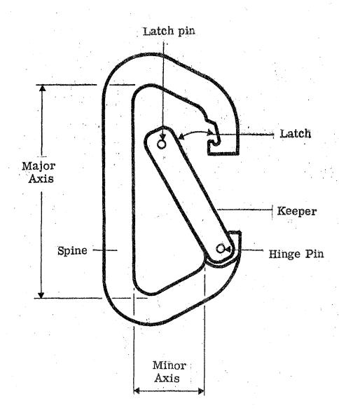
Fig.1. The parts of a typical karabina.
